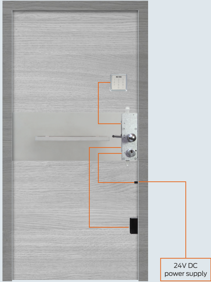
Powered by rechargeable batteries through the "Door Status Device"
